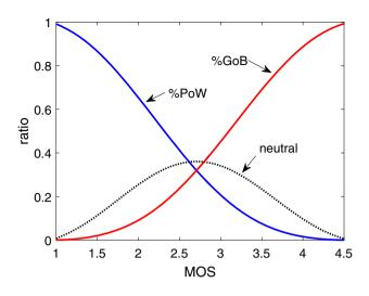
Fig. 4 Relationship between MOS, %PoW and %GoB as used in the E-model (ETSI 1996). The ratio of users not rating poor or worse as well as good or better is referred to as 'neutral' and is computed by 1-%GoB-%PoW
