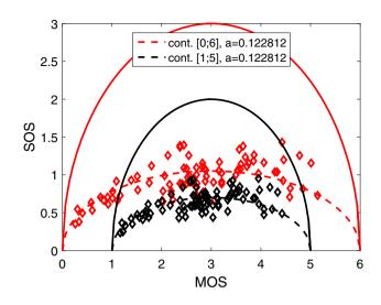
**Fig. 16** Transformation of user ratings from speech QoE results from rating scale [0; 6] to rating scale [1; 5] leads to the same SOS parameter *a*. However, the values of MOS and SOS (tuple depicted as diamond marker) as well as the maximum SOS for a given MOS (*solid lines*) are changing of course.
