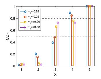
Fig. 2 Different discrete distributions with identical mean (3.5) and standard deviation (0.968). It can easily be seen that e.g. the median (and other important quantiles, in fact) are significantly different in each distribution
