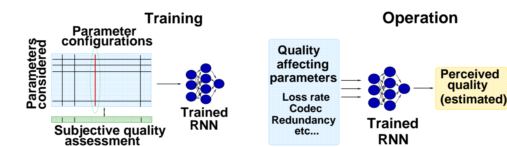
FIGURE 3: PSQA. The results of a subjective test and the parameters used to create the tested samples are used to train the RNN. The trained RNN is then able to predict the perceived quality based on measurements of the parameters considered.
